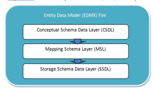
The top CSDL layer defines the entities, the bottom SSDL layer defines the database schema, and the middle MSL mapping layer aligns the CSDL and SSDL. The three layers can be exported as three free-standing XML files with file extensions .csdl, .msl, and .ssdl.
