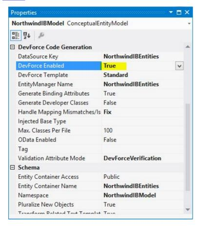
With DevForce enabled, the DevForce T4 template that guides the generation of our business model is added to SimpleStepsWeb. Notice that its name matches the name of our EDM and has the file extension "tt". If you expand the template node, you'll see a file named NorthwindIB.IB.Designer.cs. This is the code that was generated by DevForce using the template.
